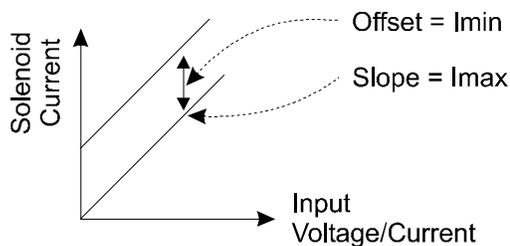
Adjusting the minimum current will shift the maximum current setting, as shown.
