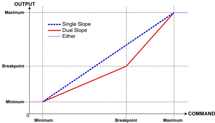
Figure 1 – Proportional Output vs. Command Profile
