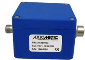
AX060003, Dual Axis Inclinometer, +85°...-85° for each axis, CANopen®, 2 M12-5 pin Connectors
