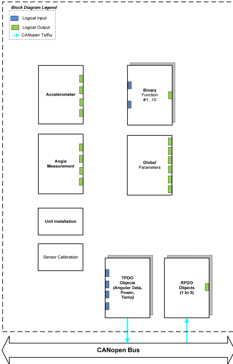
Figure 1. The Inclinometer Logical Block Diagram
