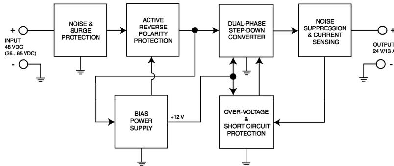
**Application:** Designed to interface between 48V batteries and 24V electrical systems such as 24V solenoids, relays and other electrical systems.
