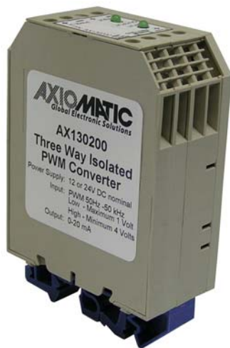
PWM to Current Signal Converter Model: AX130200
