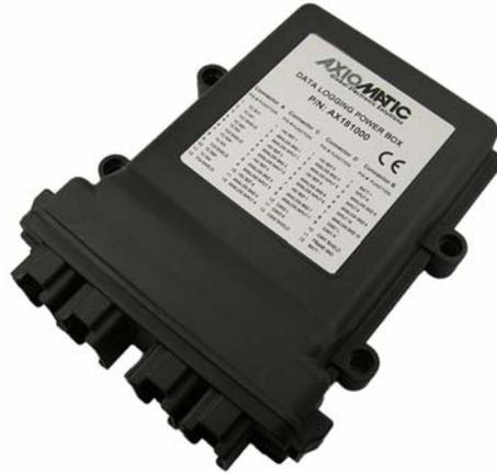
A rugged power supply interface accepts 12 Vdc, 24 Vdc or 48 Vdc nominal for battery powered machine applications. The unit carries an IP67 rating. It has a CE mark for EMC and RoHS compliance. The rugged enclosure with four 12 pin Deutsch IPD connectors is suitable for diesel engine environments. It operates from -40 to 85°C (-40 to 185°F).
