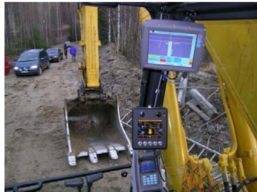
Operator display (middle) from the Axiomatic Bucket Position System shows real-time bucket position.
