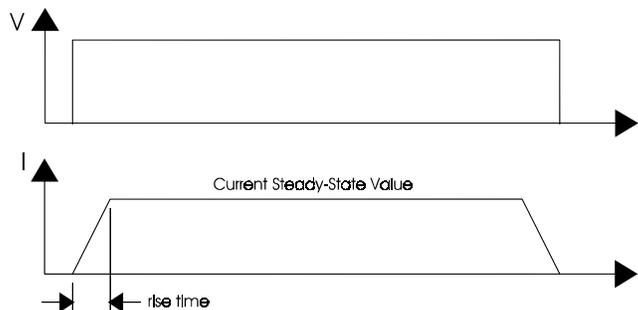
Figure 2 - Continuous Voltage Across an Inductor
