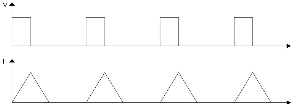
Figure 4 - Low Frequency PWM with  $D > \text{rise time}$  Resulting in Continuous Current with Ripple
