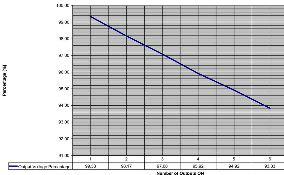
Figure 3.0 - % Output Voltage vs. No. of Outputs ON
