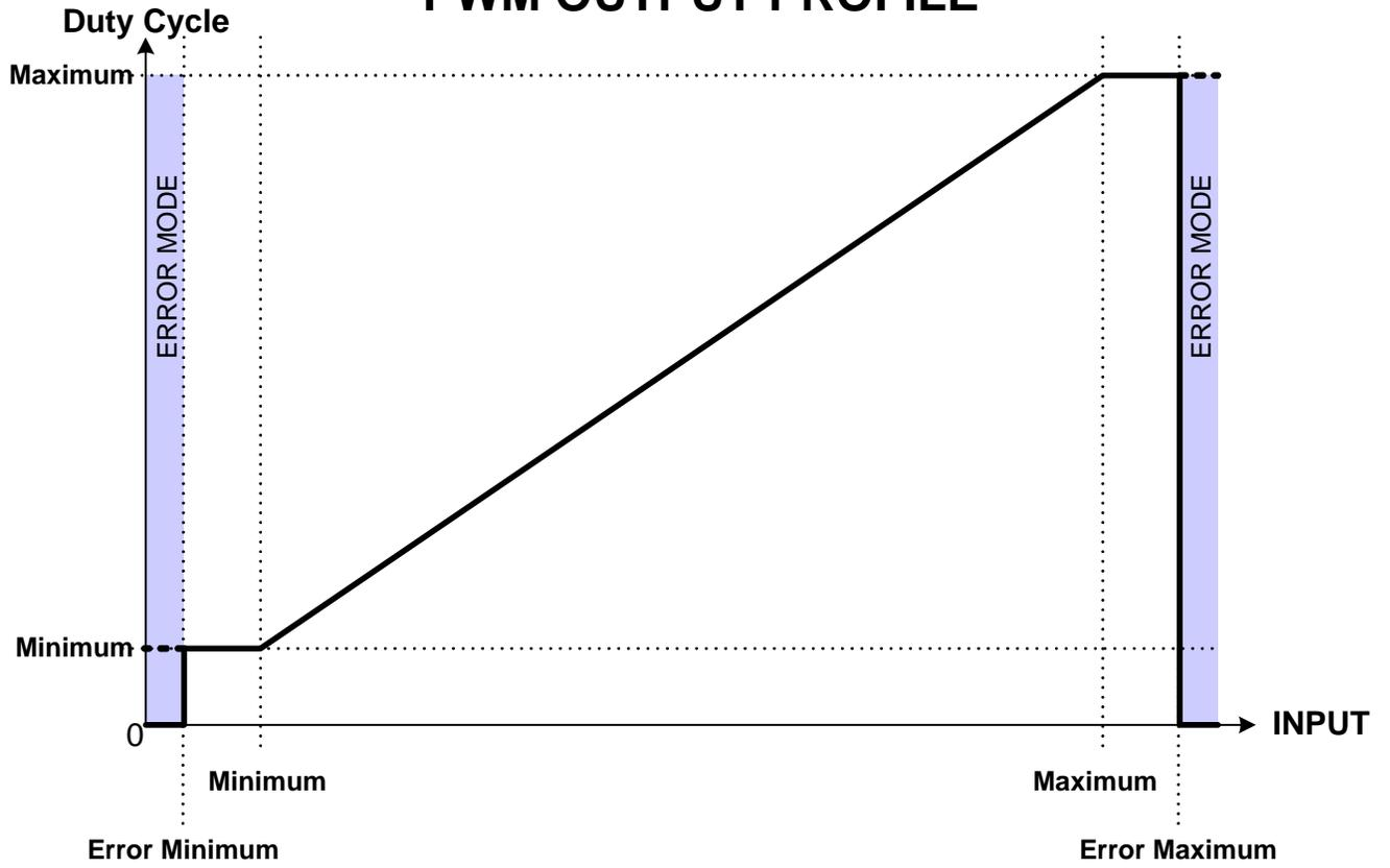
Figure 2: PWM Duty Cycle vs. Input
