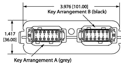
Mating Plug Assemblies for 24-pin receptacle:
