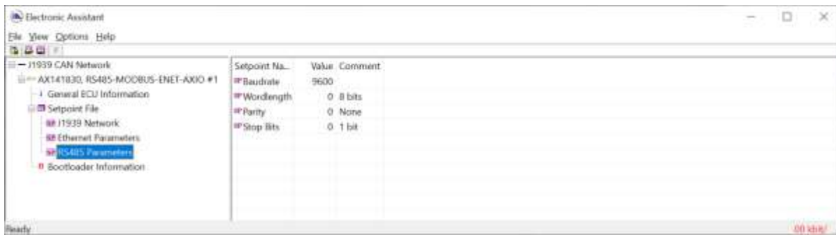
Figure 5 – Screen Capture of RS485 Parameter Setpoints
