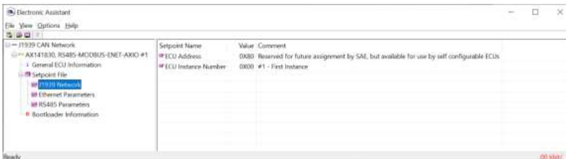
Figure 3 – Screen Capture of J1939 Setpoints
