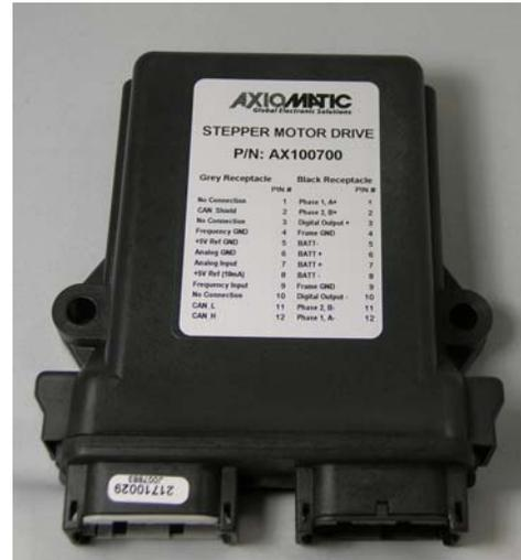
For rugged machine applications, it features the Deutsch IPD EEC-345XB enclosure and 24-pin connector. It operates with 12 or 24VDC power with surge, over and under voltage protection for battery powered devices.
