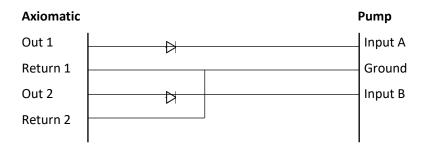
$\bowtie$  The Diode is placed here.
