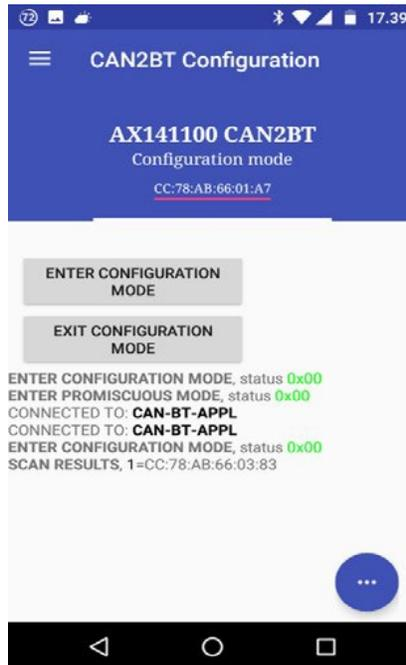
9. From the scan results, please check which entry corresponds to the Bluetooth address of the slave unit. Then, in the "CONNECTION OPTIONS" menu, use the "SET AUTOCONNECT" function and specify the node number that corresponds to the slave AX141150 device from the scan results list.
