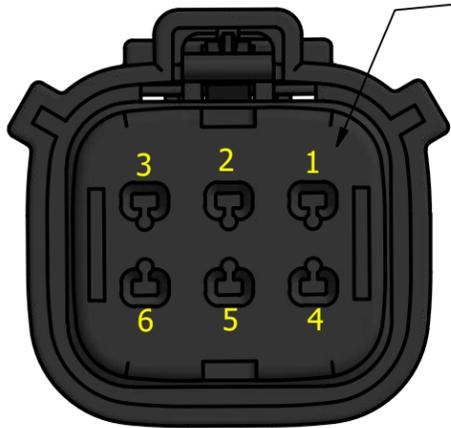
PIN 1: OUTPUT - [2M[6.5ft] 14AWG UNTERMINATED LEAD WIRE, WHITE-BLACK COLOR]
