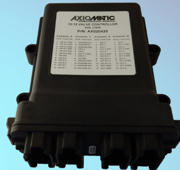
12I/12O Rugged AX020420 (SAE J1939) and AX020421 (CANopen®)
