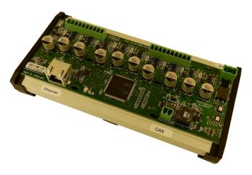
This DIN rail mount controller is operational from -40 to +85 °C and is designed to be applied in industrial process equipment. Protections on this unit include reverse polarity protection, surge and transient protection, under voltage protection, and over voltage shut down.
