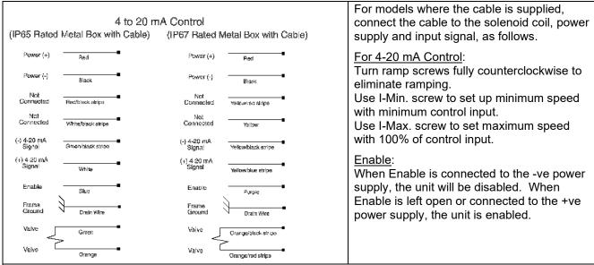
Refer to page 2 (block diagram) for an alternative method of connecting a current loop transmitter to provide a current control signal input. In this method, the current loop transmitter receives power from the power supply powering the amplifier. The transmitter is connected to the amplifier's +power supply input wire and the +4 to 20mA input wire. This method does not use the -4 to 20mA input signal wire connection.
