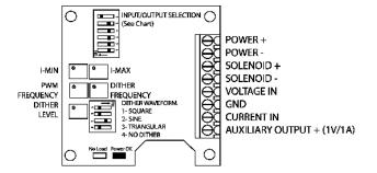
Adjusting the minimum current will shift the maximum current setting, as shown.
