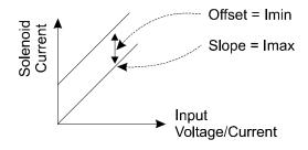
Adjusting the minimum current will shift the maximum current setting, as shown.
