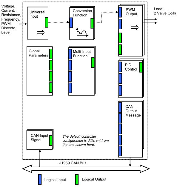
As an example, the Universal Input is connected to a Conversion Function block and the Conversion Function block is connected to a PWM Output block, providing a path for the input signal from input to output through the Conversion Function.
