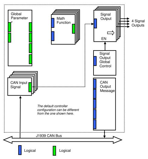
As an example, the logical output of the CAN Input Signal functional block is connected to the logical input of the Analog Signal Output functional block, providing a direct path for the CAN input signal to the controller signal output.
