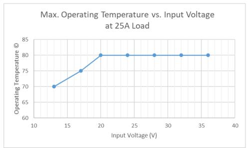
Figure 3.0 Max. Operating Temperature vs. Input Voltage at 25A Load
