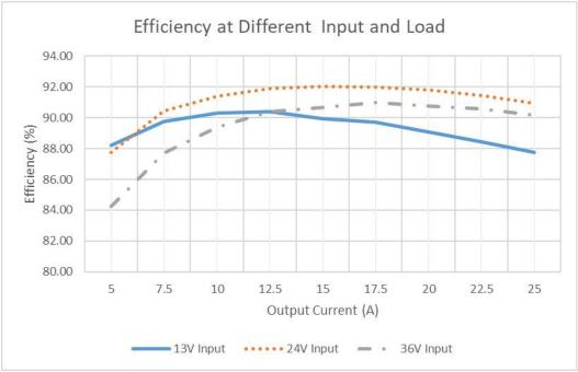
Figure 2.0 Efficiency at Different Input and Load.
