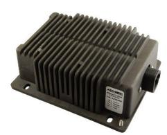
**Applications:** Designed to interface between 48Vdc batteries and 13.8Vdc electrical systems such as solenoids, relays and other electrical systems found on mobile equipment, lift trucks and buses.
