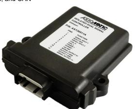
A rugged power supply interface accepts 12 or 24 VDC nominal for battery powered machine applications. The unit carries an IP67 rating. The rugged enclosure with an integrated TE Deutsch 12-pin connector is suitable for harsh environments. It operates from -40 to 85  $^{\circ}$ C (-40 to 185  $^{\circ}$ F). The powerful control algorithms allow the user to program the controller for a wide range of applications without the need for customer software.
