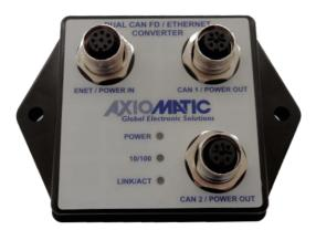
All types of Classic CAN and CAN FD frames are supported. CAN FD ports can operate either in ISO or in Bosch frame format in the Flexible Data-rate (FD) mode. Power can be passed through to the CAN port connector. Protection is provided.
