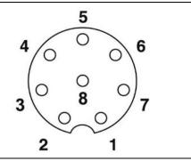
Use A-coded mating connectors compliant with IEC 61076-2-101:2012. P/N **AX070531** Ethernet and Power Cable - 1.7 m (5.5 ft.), 8-pin M12 A-coded, Unterminated Leads, Ethernet Jack, can be used for experimenting. The cable is rated for  $-40^{\circ}$ C to  $75^{\circ}$ C.
