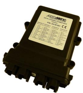
A rugged power supply interface accepts 12 Vdc, 24 Vdc or 48 Vdc nominal for battery powered machine applications. The unit carries an IP67 rating. It carries a CE mark. The rugged enclosure with four 12-pin connectors (which are TE Deutsch equivalents) is suitable for diesel engine environments. It operates from -40 to 85°C (-40 to 185°F).
