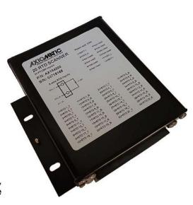
The RTD Scanner features rugged packaging and watertight connectors for an IP67 rating. The connectors are TE Deutsch equivalents. The RTD Scanner is designed to meet the environmental, EMC and vibration requirements of vehicle applications.
