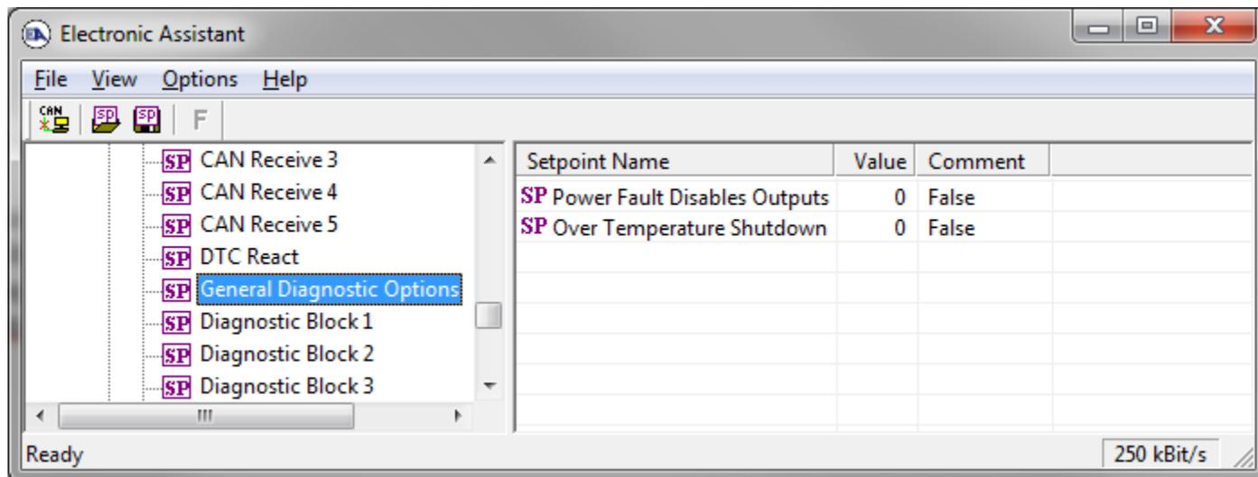
Figure 18 - Screen Capture of General Diagnostics Options Setpoints
