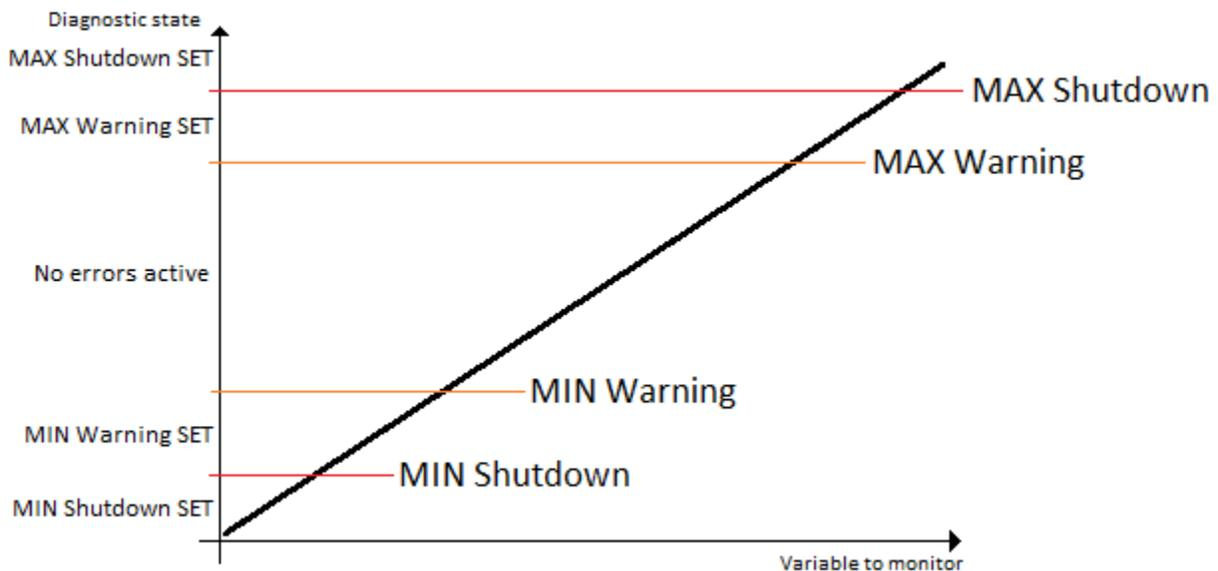
**Figure 3 – Double Minimum and Maximum Error Thresholds**
