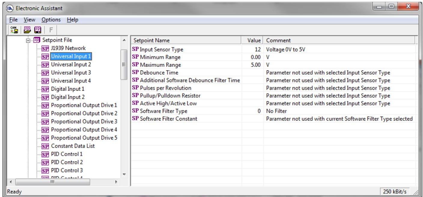
Figure 7 - Screen Capture of Universal Input Setpoints
