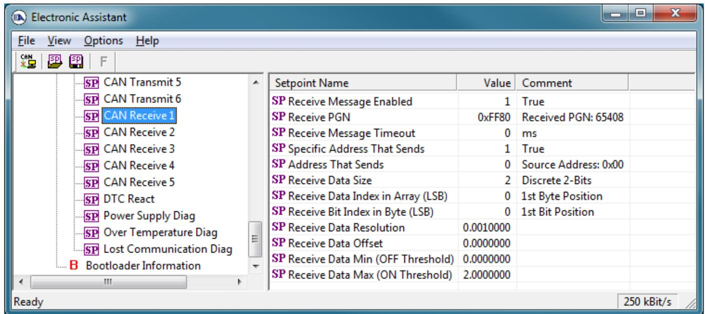
**Figure 16 - Screen Capture of CAN Receive Message Setpoints**
