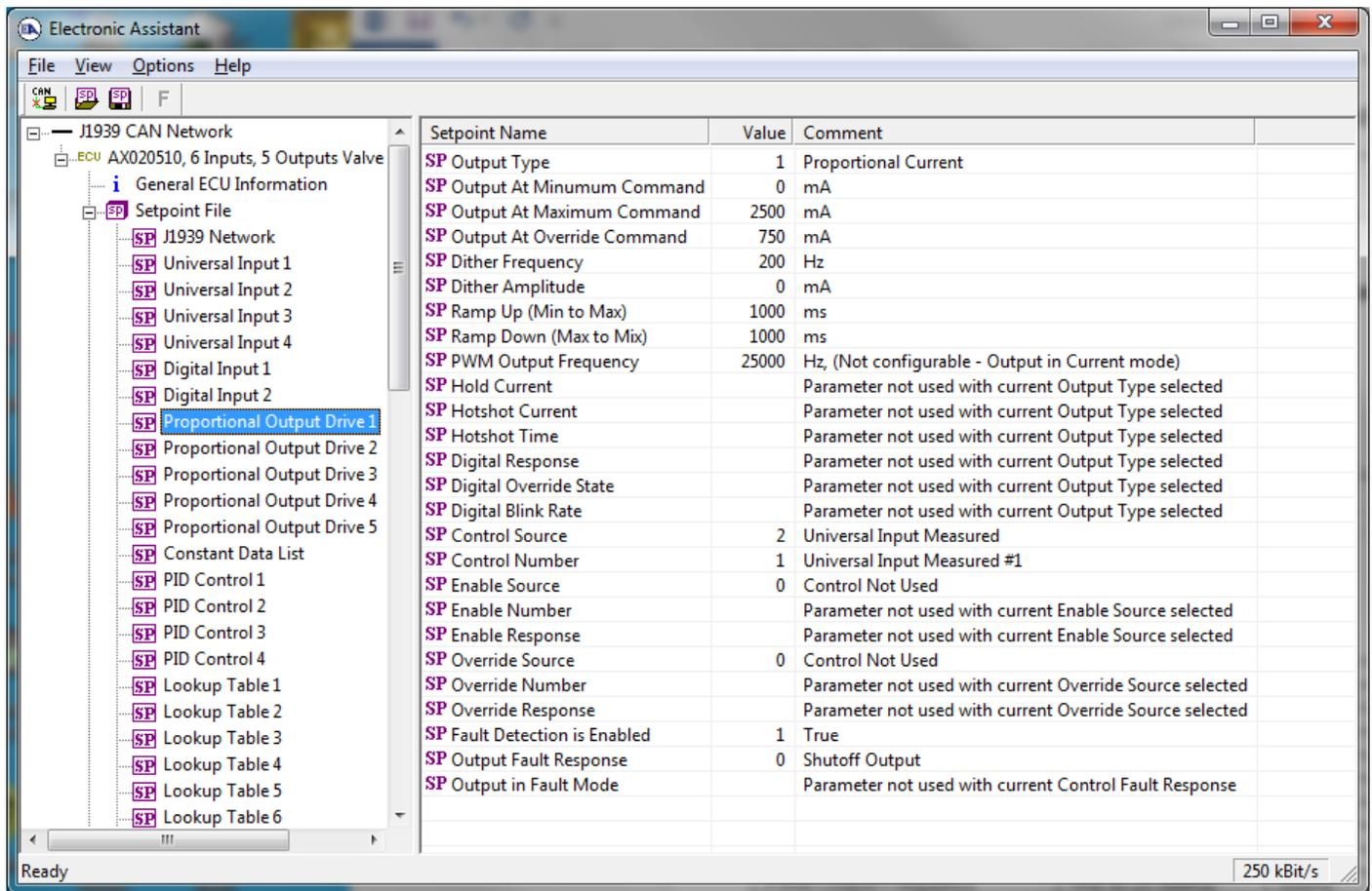
Figure 9 - Screen Capture of Proportional Output Setpoints
