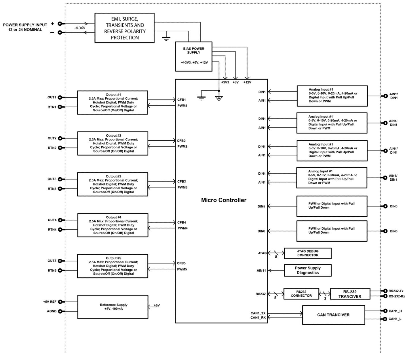
**Figure 1 - AX020510 Block Diagram**
