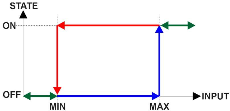
**Figure 4 - Analog source to Digital input**
