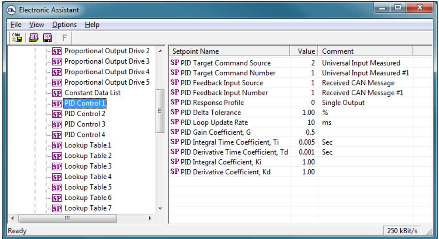
**Figure 11 - Screen Capture of PID Control Setpoints**
