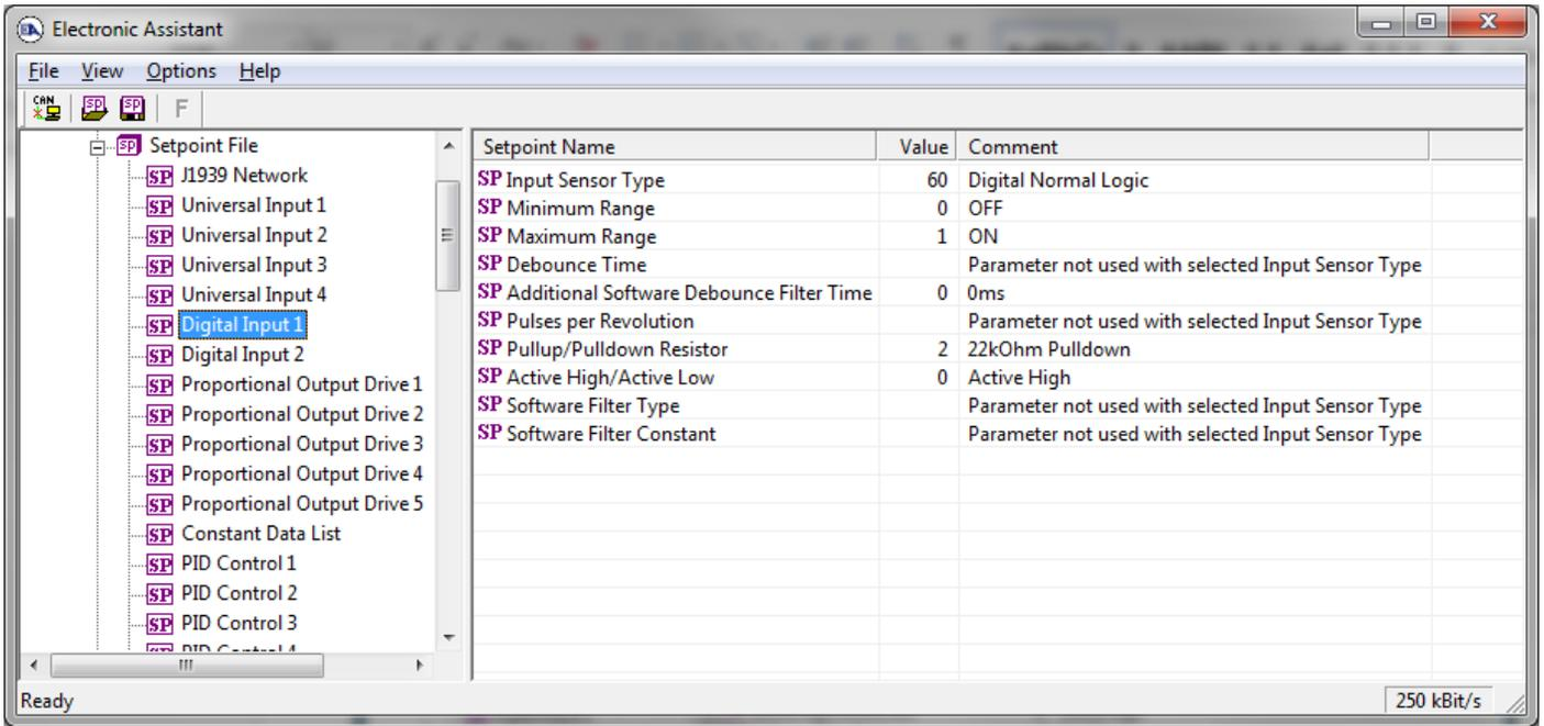
**Figure 8 - Screen Capture of Digital Input Setpoints**
