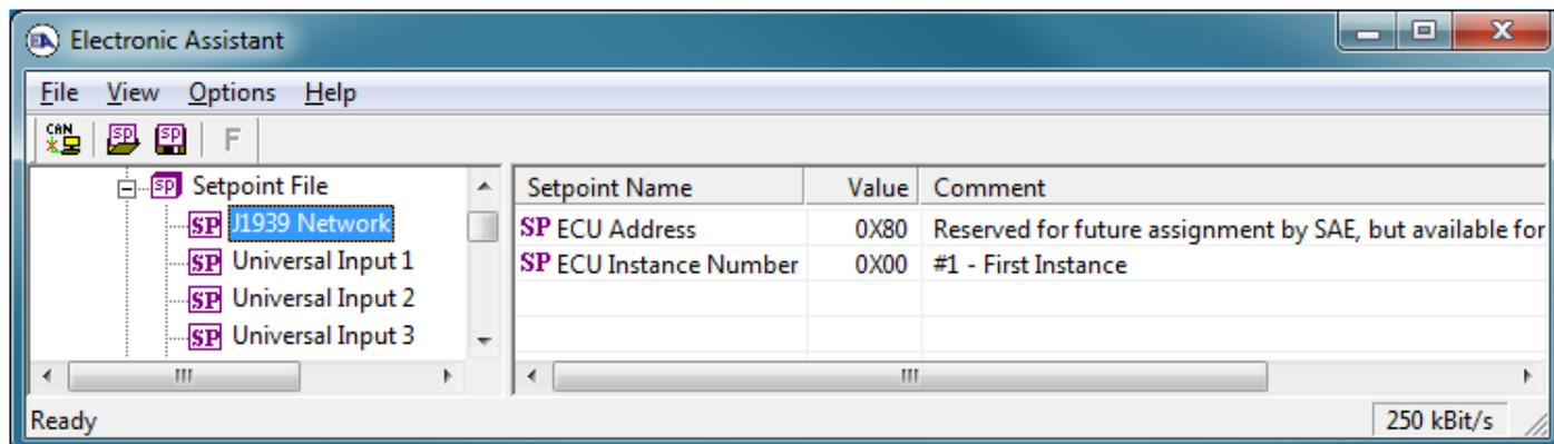
**Figure 6 - Screen Capture of J1939 Setpoints**
