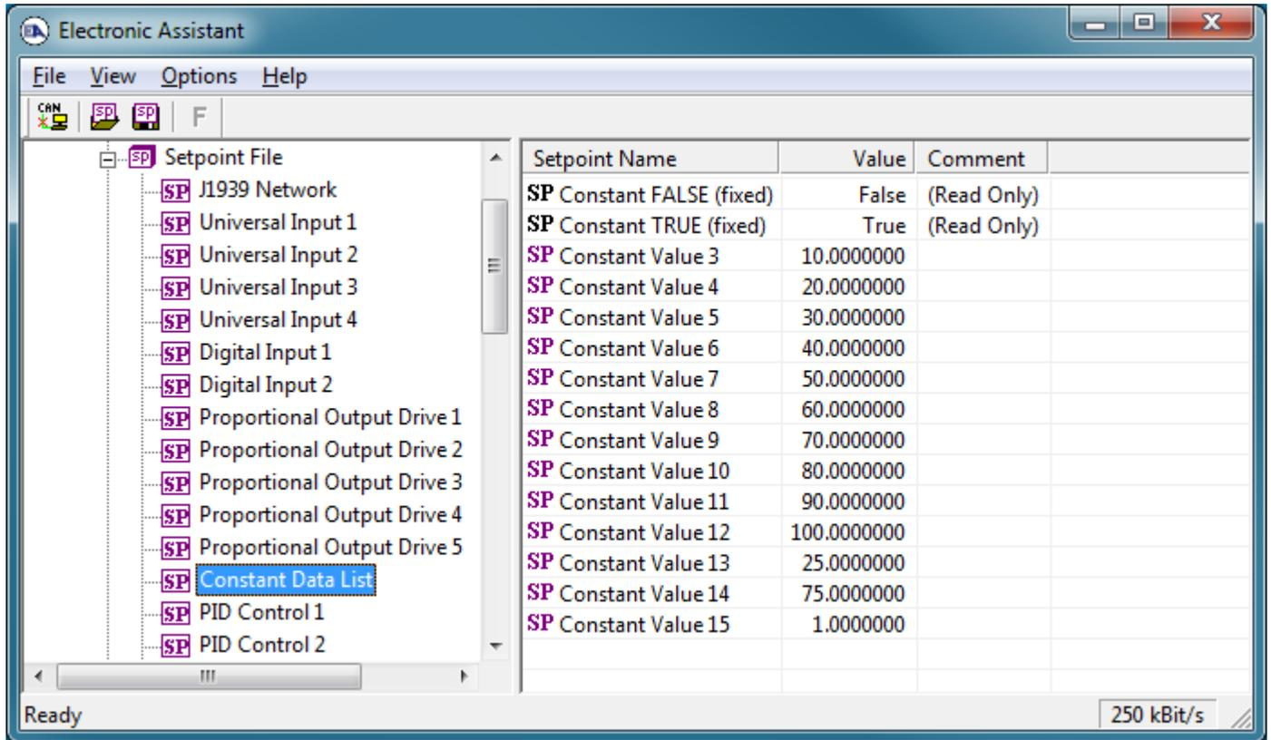
Figure 10 - Screen Capture of Constant Data List Setpoints
