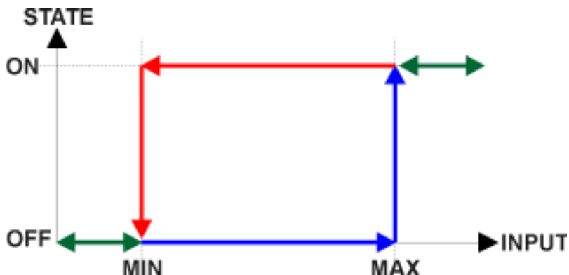
Figure 5 – Analog Input Read as Digital
