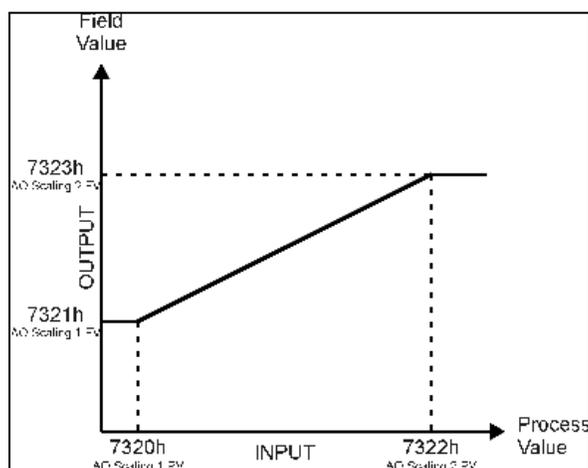
**Figure 11 – Analog Output Linear Scaling PV to FV**
