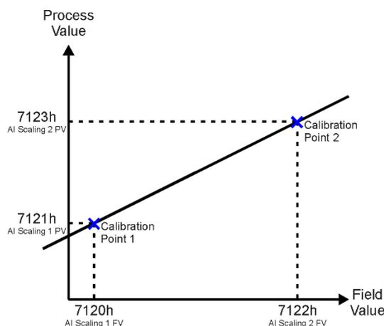
**Figure 8 – Analog Input Linear Scaling FV to PV**
