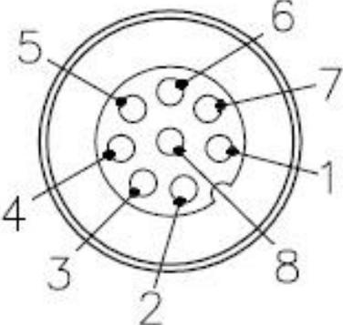
Use A-coded mating connectors compliant with IEC 61076-2-101:2012.
