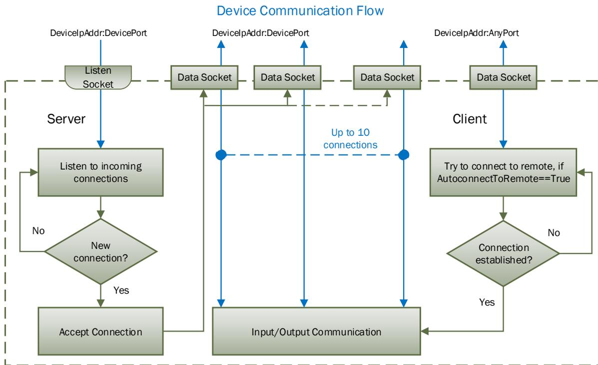
Figure 4. Communication Device. TCP Protocol
