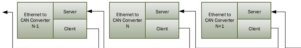
Figure 25. Daisy-Chain Converter Connection
