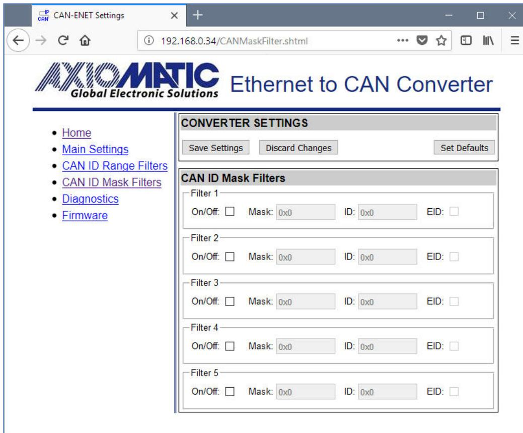
Figure 13. Converter CAN ID Mask Filters Page
