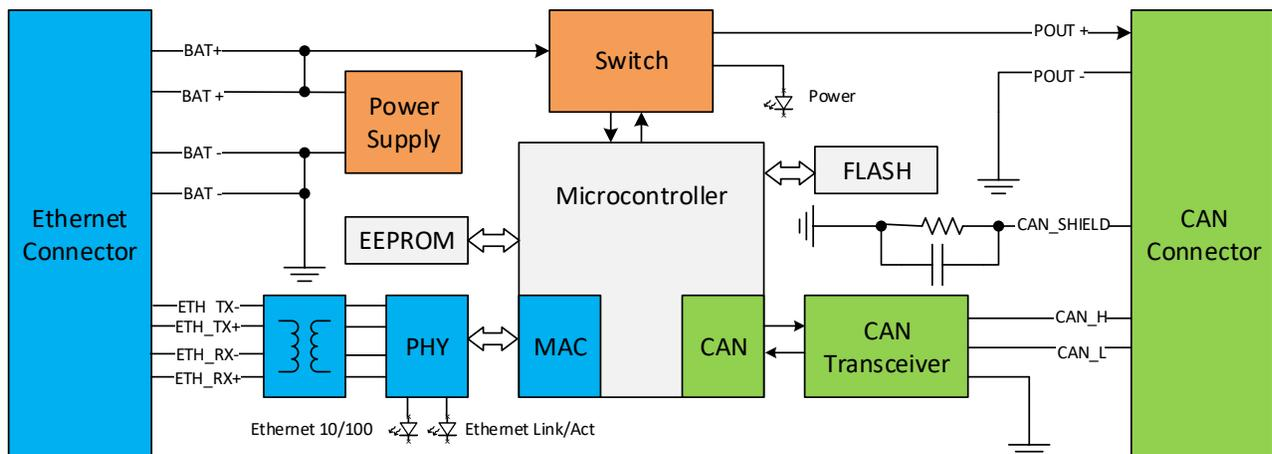
Figure 1. The Converter Hardware Block Diagram
