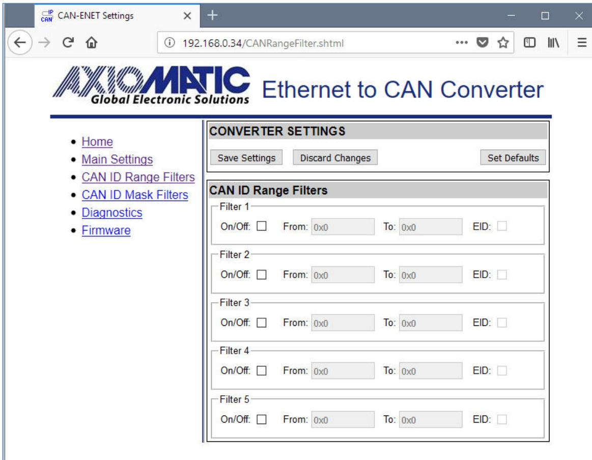
Figure 12. Converter CAN ID Range Filters Page
