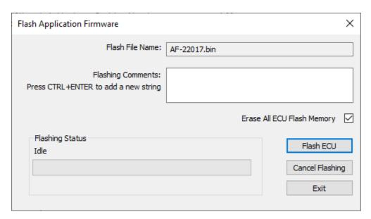
**NOTE:** If the "Erase All ECU Flash Memory" box is checked, all configuration data currently stored in non-volatile flash including PIN codes will be deleted.
