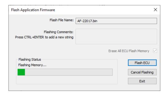
Once the firmware has finished uploading, a message will pop up indicating the successful operation. If you select to reset the ECU, the new version of the AX141155 application will start running, and the ECU will be identified as such by the Axiomatic EA. Otherwise, the next time the ECU is power-cycled, the AX141155 application will run rather than the bootloader function.
