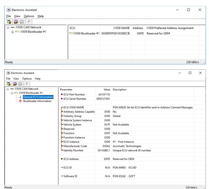
Note that the bootloader is NOT Arbitrary Address Capable. This means that if you want to have multiple bootloaders running simultaneously (not recommended) you would have to manually change the address for each one before activating the next, or there will be address conflicts. And only one ECU would show up as the bootloader. Once the 'active' bootloader returns to regular functionality, the other ECU(s) would have to be power cycled to re-activate the bootloader feature.
