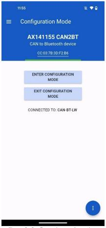
Figure 2- Configuration mode settings
