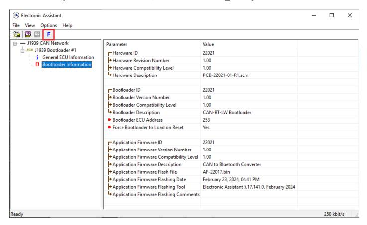
6. Select the <u>F</u>lashing button and navigate to where you had saved the **CAN2Bluetooth.bin** (or equivalent) file sent from Axiomatic. (Note: only binary (.bin) files can be flashed using the Axiomatic EA tool.)
