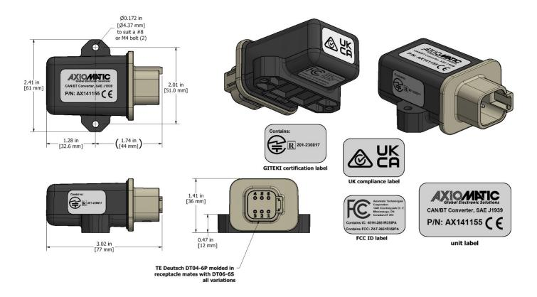
Figure 10 – AX141155 Dimensional Drawing
