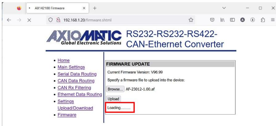
The firmware upload process is shown below the 'Upload' button.
