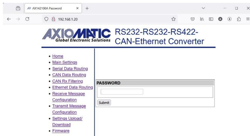
When the correct password is entered, the configuration page is opened. The settings can be applied by clicking the button at the top of the page. In case the user doesn't want to change settings, the connection can be closed.
