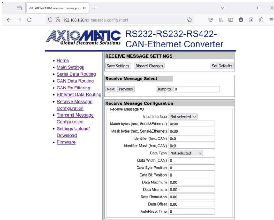
A value from a received frame, such as GPS data, can be parsed using the configuration options available in the Receive Message Configuration page. 3RS-ENET-CAN converter supports 4 serial message configurations.
