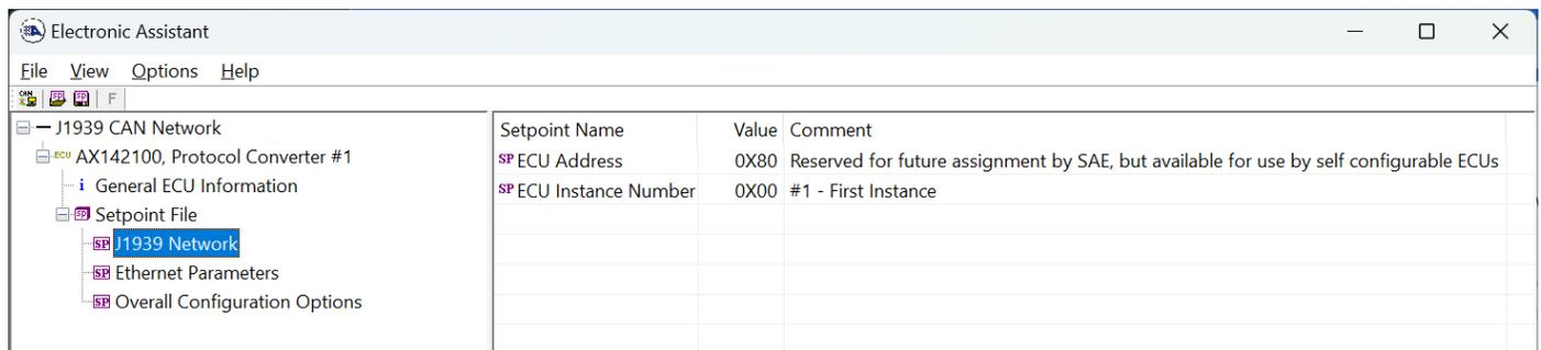
Figure 4 – Screen Capture of J1939 Network Setpoints
