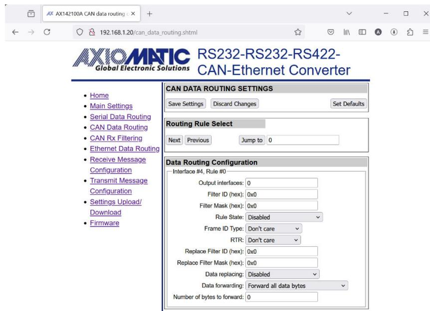
CAN interface supports 16 data routing rules. Each one of the rules has a list of **Output interfaces**, **Filter ID (hex)** and **Filter Mask (hex)** (software filter) and Data replacing options. The data replacing is supported for the CAN Frame ID bits. Also, the number of data bytes to forward can be specified.
