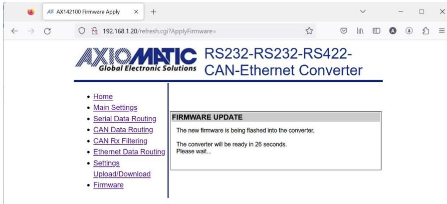
The firmware reflash procedure takes 30 seconds to finish. After this the AX142100A reboots automatically to the new firmware and returns to the password dialog.
