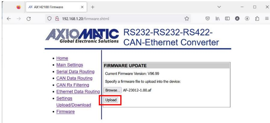
Once the file is selected, the actual upload/upgrade process is started by pressing the 'Upload' button.
