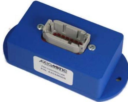
The **Fan Drive Controller Platform**, p/n **AX022600S**, accepts 2 discrete inputs, 1 Hall Effect sensor (or digital/PWM signal) input, and provides a 4A output (0-200 Hz, 50% D.C.) to drive a solenoid. The unit has a 100mA +5V reference and operates with 12 or 24VDC power. The CAN bus communication port, SAE J1939, interfaces with the engine ECM. It operates over -40 to 125°C (-40 to 257°F).
