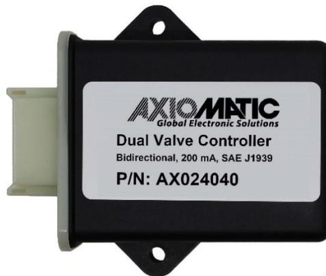
This servo valve controller can operate with battery power supply of 8 V to 36 V and is protected against reverse polarity, surge and transient, overvoltage, and undervoltage faults. The outputs have overcurrent and short circuit protection. It can work at temperatures from -40 to 85 °C (-40 to 185 °F). The sealed enclosure is rated IP67 against dust and water exposure.
