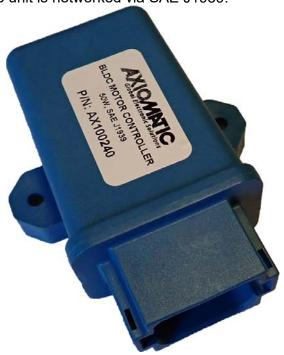
Axiomatic brushed DC motor controllers such as AX102100 operate the steer function and AX105000 operates the drive function industrial lifts. Other controllers operate tailgate lifts. Additional I/O on the controller can drive machine hydraulic functions (boom-in / boom-out), control a machine brake, and monitor sensors / switches for safety features.
