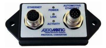
The Institute of Electrical and Electronic Engineers (IEEE) 802.3bp standard (also known as 1000BASE-T1) is a 1000 Mbps Automotive Ethernet standard aimed at increasing data throughput, meeting strong automotive emissions standards, and reducing cabling weight and cost in automotive networking. Automotive Ethernet networks use a 2 wire, unshielded, twisted pair (UTP) cable.
