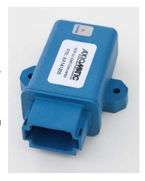
CAN frames are converted into UDP or TCP IP datagrams, and vice versa, sending them over a wireless network using a Wi-Fi protocol. The AX141200 Wi-Fi connection is provided by an internal antenna. The Wi-Fi port can work in a station or access point mode in 2.4GHz or 5GHz frequency range.
