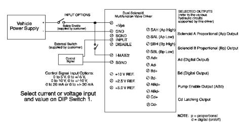
Multiple outputs are available to support a variety of hydraulic circuits as described on page 2. The diagram below shows the outputs from the Dual Solenoid Multifunction Valve Driver as a reflection of the movement of a remote joystick. The electronic joystick deadband (Setting 5 on Switch 2) was selected.
