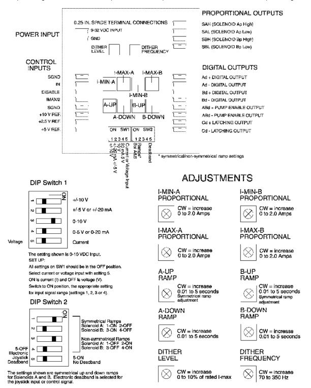
Adjustments to the single turn potentiometers are made using a flat head or Philips screwdriver. For P/N: DSDA-SMB-SC-MT-1A, minimum and maximum current adjustments are 20 turn pots.
